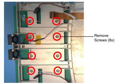
Figure 6.12 DTC Nest Frame removal
