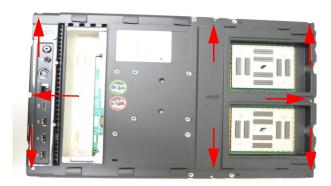
Figure 6.4 Base Assembly Screw Removal
