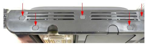
Figure 6.1 Screw Cap Removal
