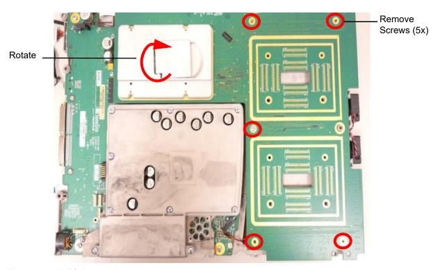
Figure 6.13 DTC Removal
