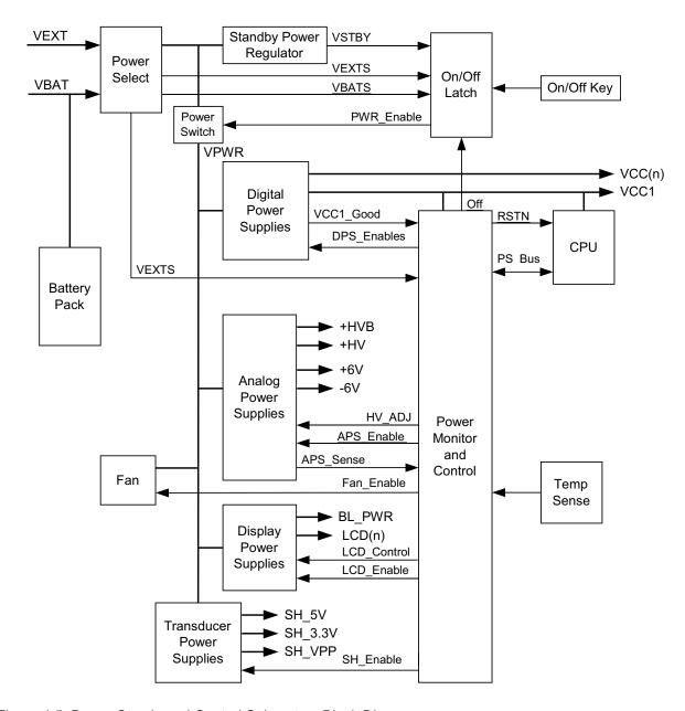
Figure 4.5 Power Supply and Control Subsystem Block Diagram
