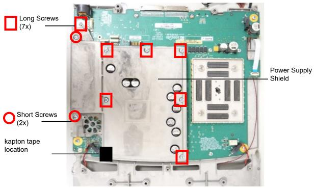
Figure 6.16 Power Supply Shield
