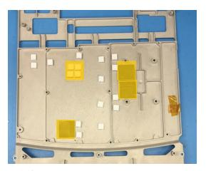
Figure 6.21 Thermal Pad placement
