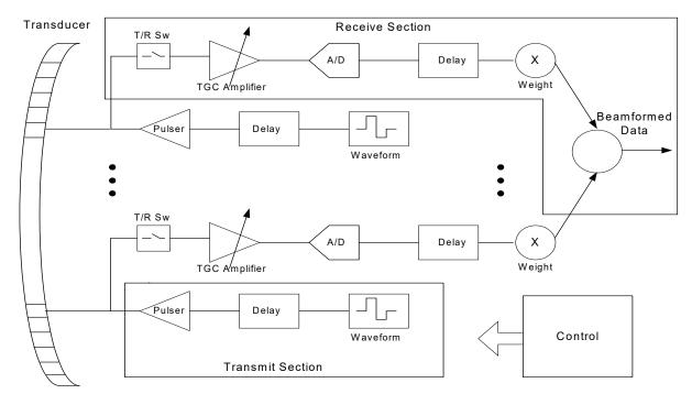
Figure 4.2 SII Front End block diagram
