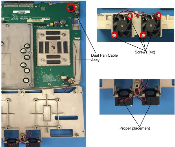
Figure 6.15 Dual Fan Removal
