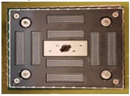
Figure 6.18 Turbo System Interposer Assembly
