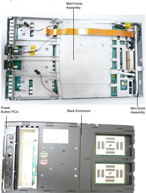
Figure 6.8 Base Assembly top and bottom
