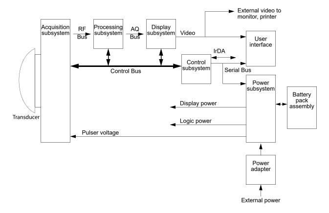
Figure 4.1 SonoSite SII High-Resolution Ultrasound System Block Diagram
