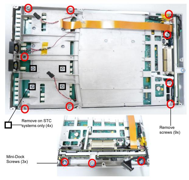
Figure 6.10 Back Enclosure Removal
