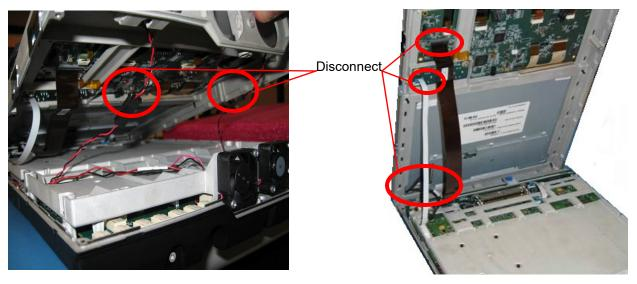
Figure 6.5 User Interface Removal
