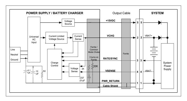
Figure 4.6 Battery Charging Subsystem Block Diagram
