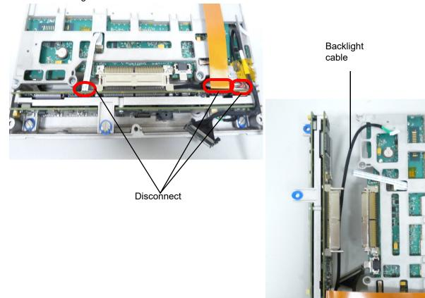
Figure 6.11 Internal Mini-Dock Removal
