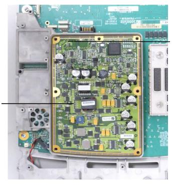
Power Supply connector underneath mates Power Supply PCBA to the Main PCBA.
